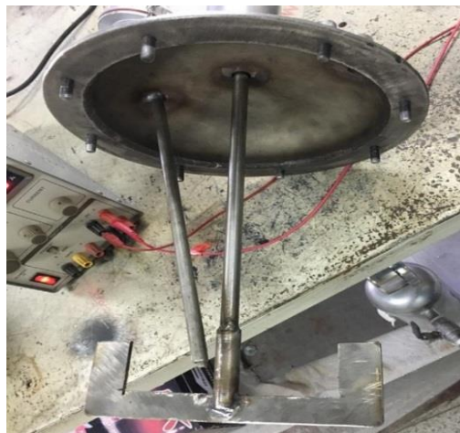
Fig. 2. An Anchor stirrer was installed inside the digester
