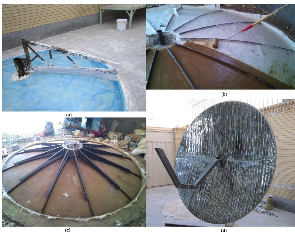
Fig. 3. PD Concentrator Fabrication Steps: (a) Gypsum Mold; (b) Layering With Needle Felt and Polyester Resin; (c) Dried Product; (d) Mirrored Dish
