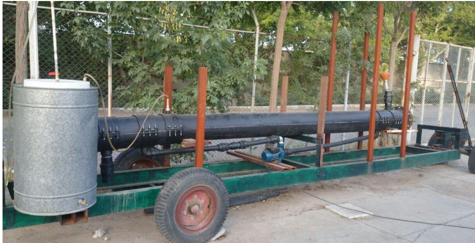
Fig. 2. Assembled portable polyethylene-based biogas reactor located at the Ferdowsi University of Mashhad, Iran
