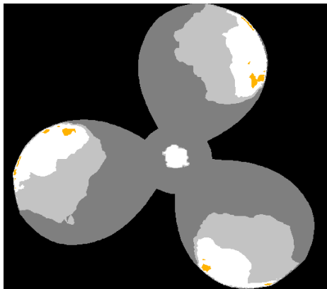
Fig. 15. The volume fraction of the vapor over the blades in j = 0.6
