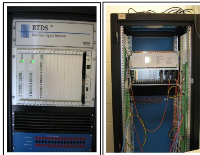
Fig. 1. RTDS front and back panels
