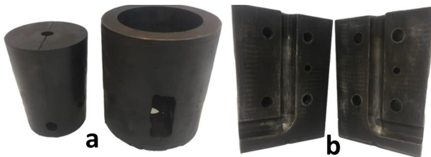
Fig. 2. The ECAP die components, a) general view, b) disassembly view
