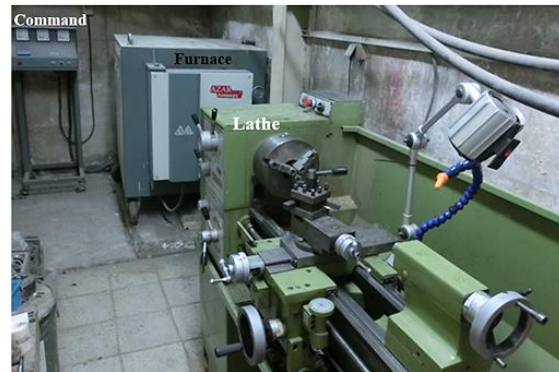
Fig.2: Lathe and furnace used for hot turning
