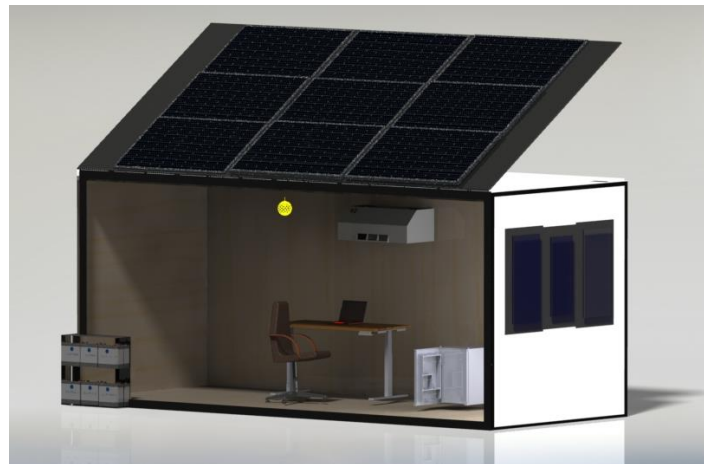
Fig. 1. Proposed Conex with its off-grid PV system
